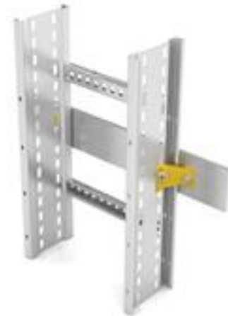
Safe working load 215kg per pair of adaptable fixing brackets when supporting Speedway cable ladder installed as part of a vertical run
