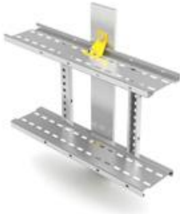
Safe working load 300kg per pair of adaptable fixing brackets when supporting edge mounted Speedway cable ladder
